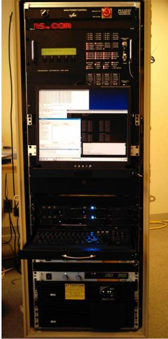
The Integrated Test Rack (ITR) is a complete EGSE test suite for command and control of spacecraft and other complicated systems. The ITR is a turn-key integration and test solution with capabilities proven through rigorous spacecraft I&T campaigns. Tiger Innovations EGSE racks have been used on the HENEX program, STPSat-1 mission, and are currently being built to support the STP-SIV mission with delivery in Fall 2007.
