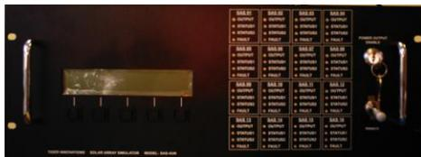
The Tiger Innovations SAS (TSAS-4UN) provides up to 16 individual solar array simulators. Each simulator is individually controllable for max-power current/voltage, short circuit current, and open circuit voltage. Additionally, each simulator has a PRTD simulator covering the range of  $-120^{\circ}\text{C}$  to  $+120^{\circ}\text{C}$ . The TSAS-4UN fully integrates with StreamLINK and can be controlled via the front panel or Ethernet.
